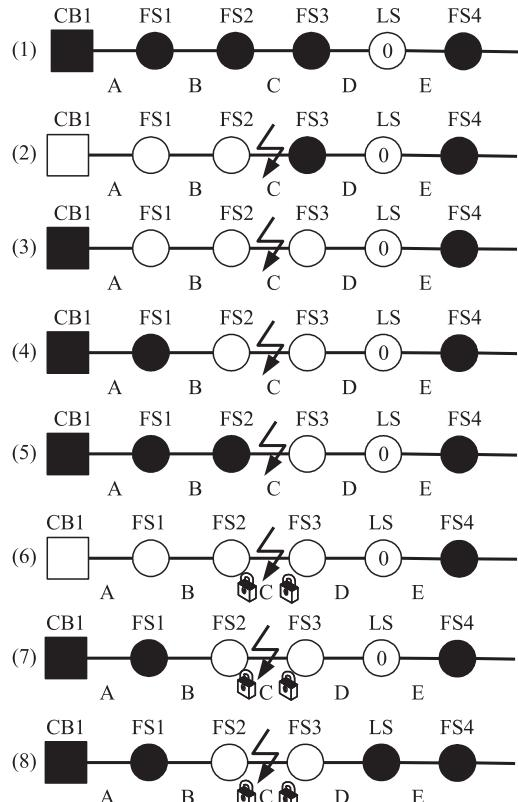
图2 故障隔离过程解析
